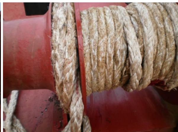
Actual ropes/drum, note that the free end is between coils approximately centre of the rope drum in the left hand picture, in the right hand picture see also loose turns caught around the drum axle which eventually stalled the electric drive motor.
