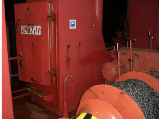
View of the exit to the forecastle space and view of the exit from the forecastle deck, the exit partially obstructs the view of the control levers from the bridge.
