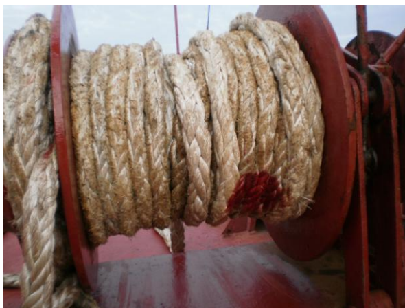
Actual ropes/drum, note that the free end is between coils approximately centre of the rope drum in the left hand picture, in the right hand picture see also loose turns caught around the drum axle which eventually stalled the electric drive motor.
