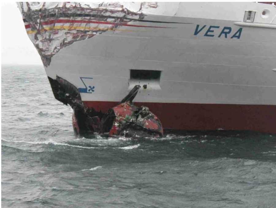
Damage to MV Vera
