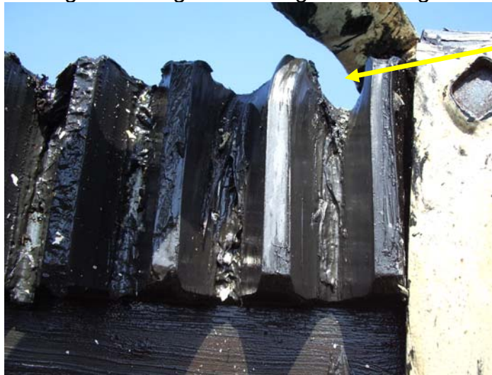
Damage to slew gear showing bent slewing gear
