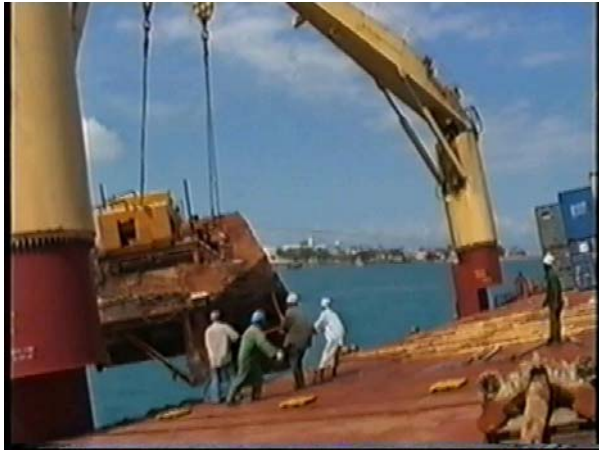
Vessels list increasing as cranes being dragged outboard by the weight of the barge. Note forward tag line, tight but not holding
