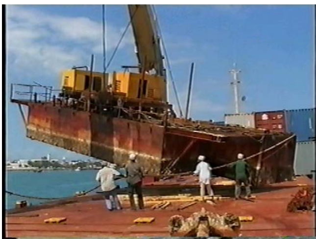
Forward end of barge twisting outboard
