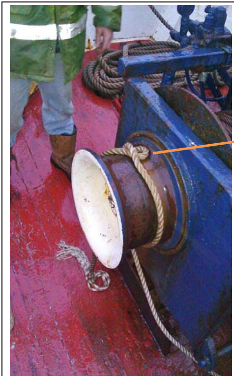
Port winch drum end
