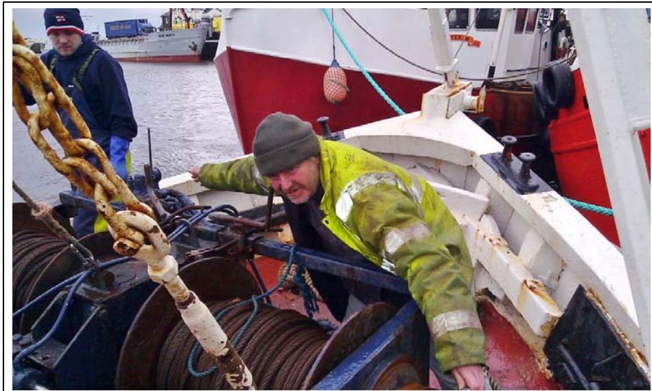
Crew member simulating working with starboard drum end, unable to reach winch operating handle
