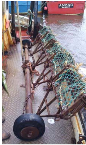
Port tow bar attached to five frames/bellies
