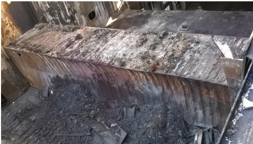
Container 700020 showing deformed side adjacent to 700220
