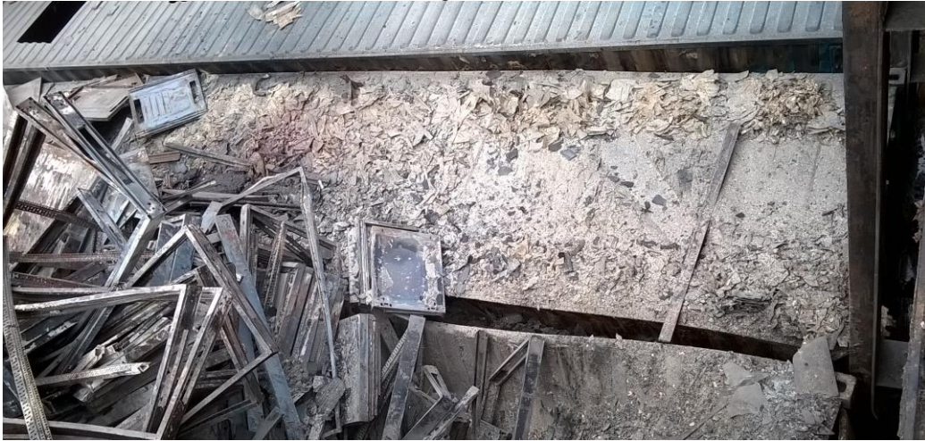
Container 700420 showing deformed side adjacent to 700220
