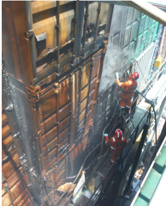
SMIT firefighters burning an access hole into a burning container
