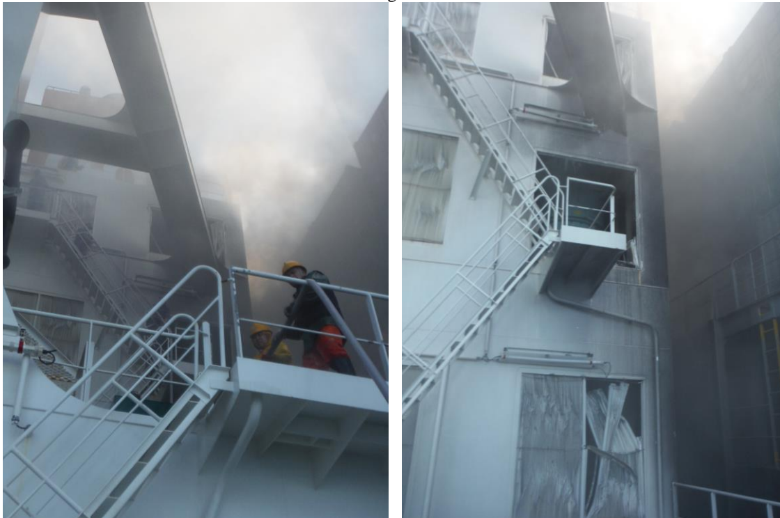
Egyptian Fire Team preparing hoses on stbd side of fan room casing and second image shows damage to the water catchers from the FiFi tug water monitors
