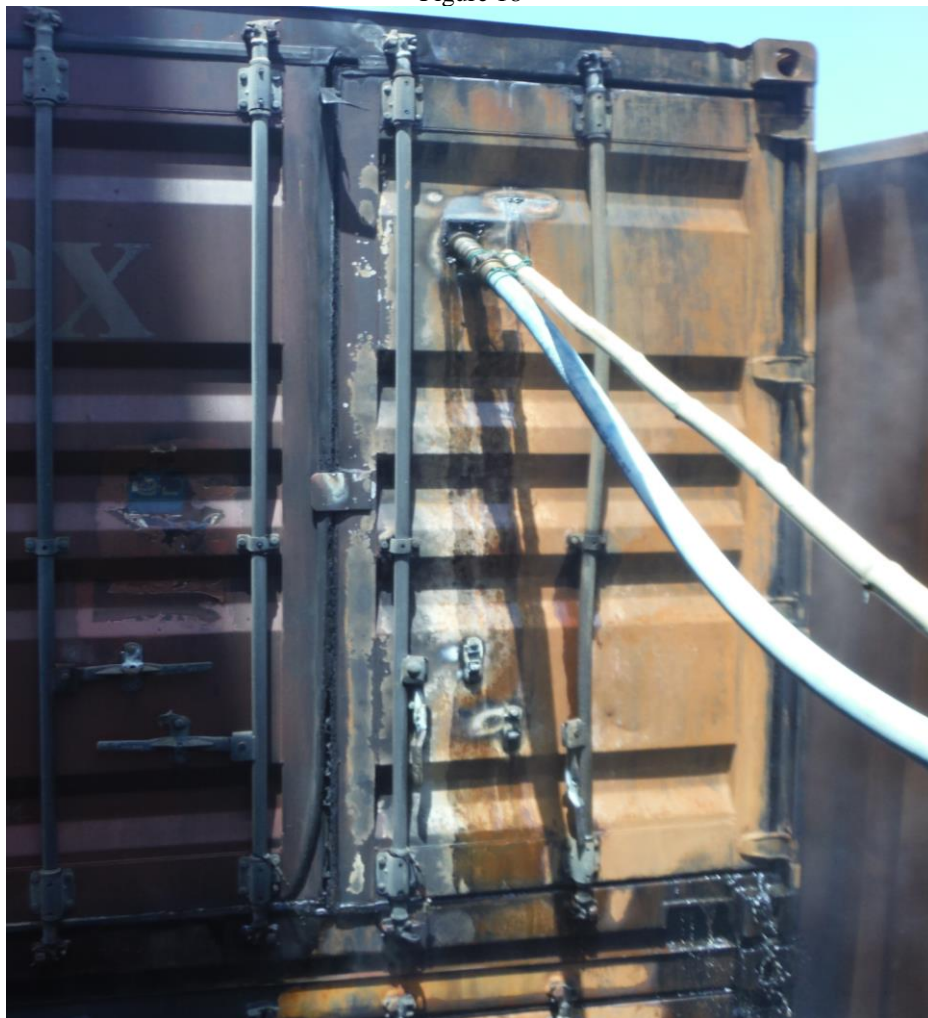
Cooling hose rigged into container aft end of bay 70 adjacent to ER casing
