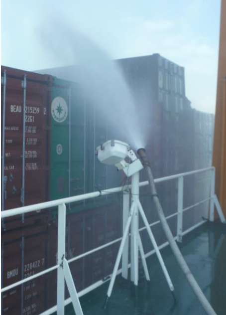
SMIT Team setting up water barriers
