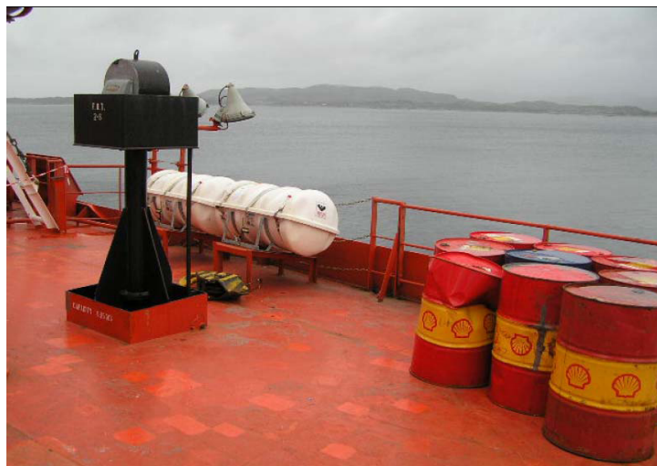
Figure of fuel oil vent pipe save-all
