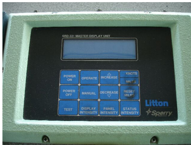
The speed log display unit installed on console B.
