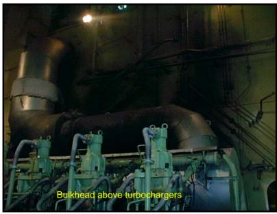
2.2 Soot was deposited over the entire side of the engine, on walkways, pipework, lagging and fittings facing the crankcase relief valves. Shadow areas (where soot was lightly deposited) existed on the ships side in way of deep frames and web frames in line of sight from the relief valves and where pipes intervened or the walkways turned back on themselves
