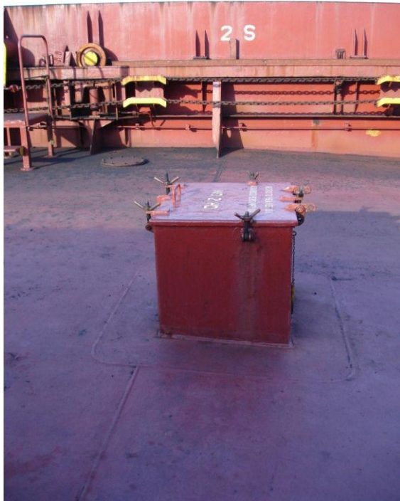
Hold #2 Aft main deck access hatch
