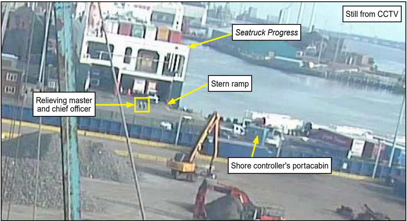
Figure 2: Stern ramp in its lowered position on the quay
