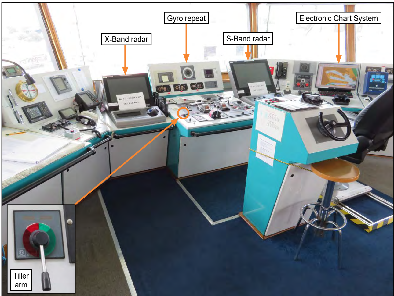
Figure 7: Central bridge area layout
