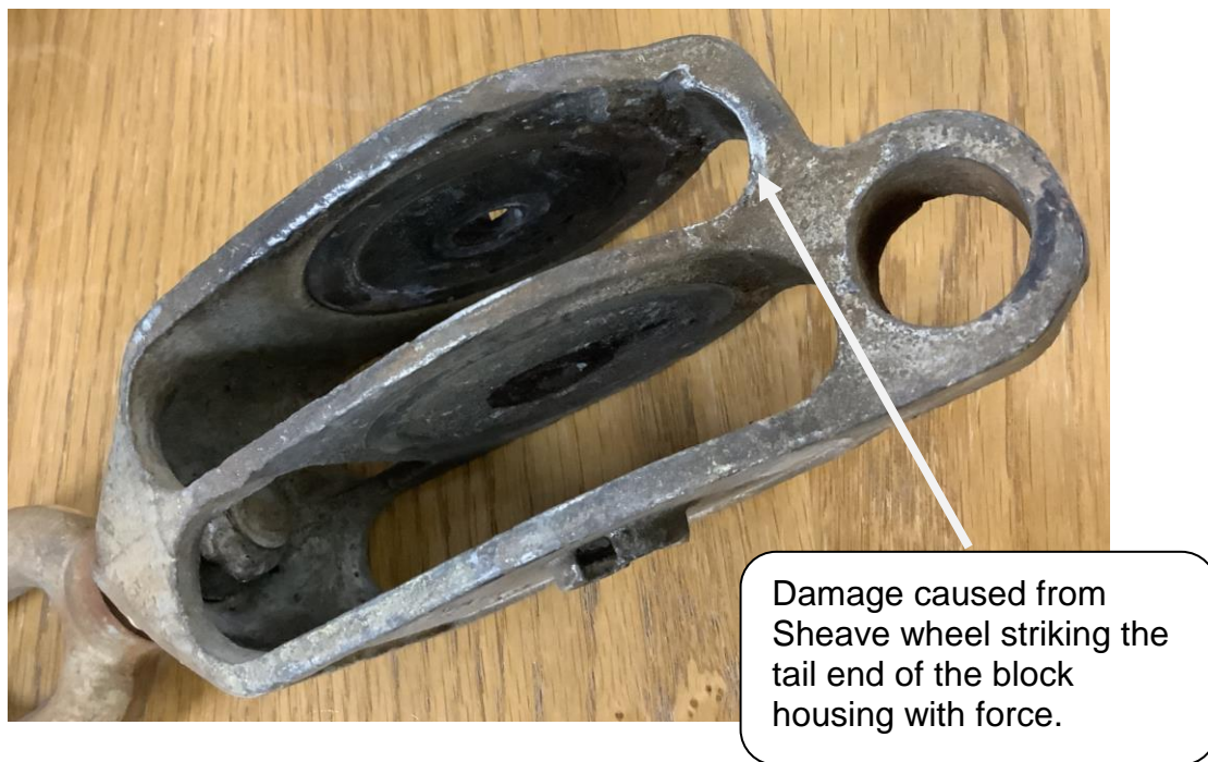
Fig 13- Damage to block housing from ejected sheave wheel
