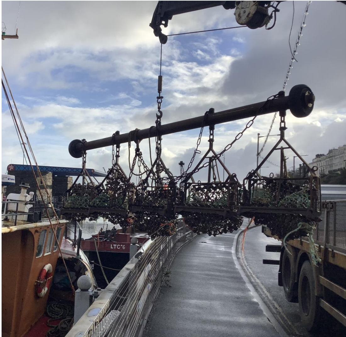
Fig 06 - Empty Port side scallop dredge gear being removed from the Silver Viking to be weighed.
