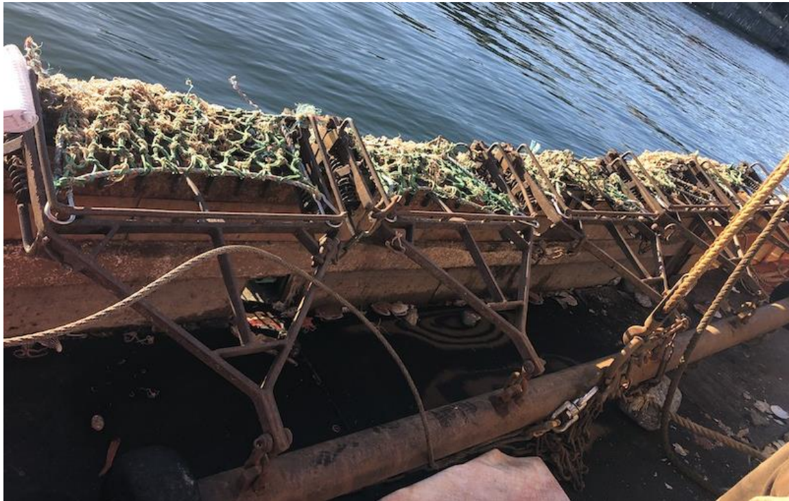
Fig 02 - dredge bar with 5 dredge nets resting on port side of the vessel.
