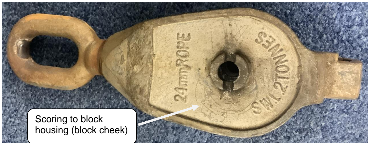
Fig - 11 – Upper hauling block from Silver Viking with block cheek scoring.
