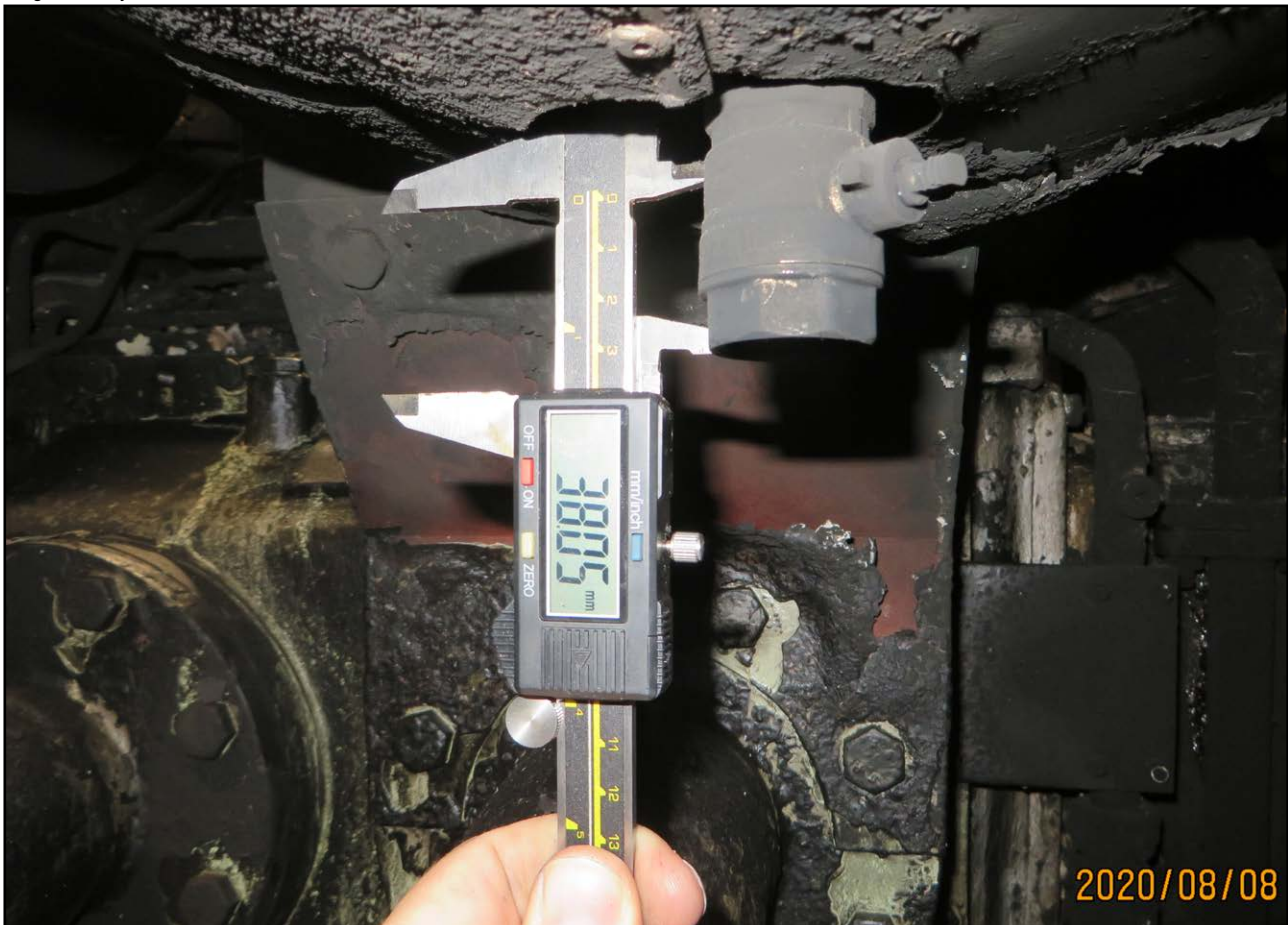
Figure 22: AE2 exposed turbocharger water washing drain connection
