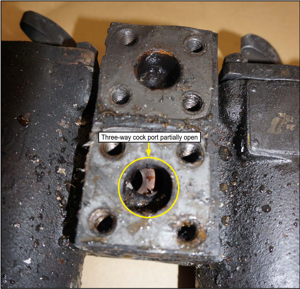
Figure 18: AE1 fuel filters three-way cock ports partially open
