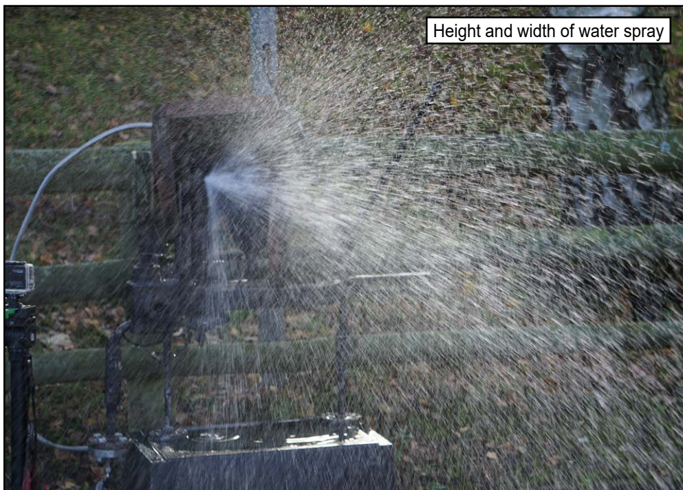
Figure 17: AE1 left-hand fuel filter leakage test
